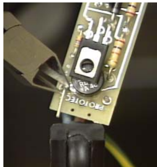
Cut off excess capacitor leads AFTER soldering.
