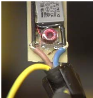
Solder power cord to capacitor leads.
