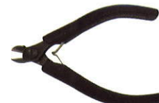
KP9550 Regular Bevel Cutter with Oval Head for Copper Wire: .015in. (.4mm) - .078in. (2mm) L: 4.9" (125 mm)
