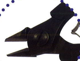
KP9356 Regular Bevel Cutter with Tapered Head for Copper Wire: .012" (.3 mm) - .049" (1.25 mm) L: 4.4" (112 mm)
