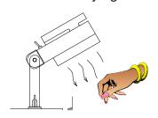
While fan assembly is turned to face the opposite direction, remove both filters for drying clients nails.
